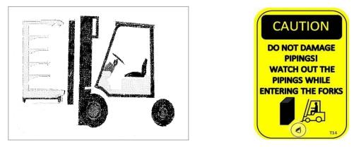
TEFCOLD Refrigeration manufactures its refrigerated cabinets suitable to be lifted using a suitable forklift. Care must be taken to place the forklift forks into appropriate areas underneath the cabinet.
