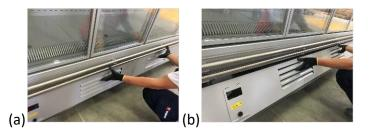
(a) - (b) Pull up the front lift off panel and then pull toward yourself. This will reveal the condenser, compressor and high & low pressure switches, all accessed from the front.
