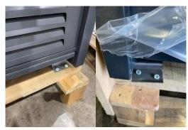
Case can now be lifted off using the correct lifting equipment. Follow the foot adjustment to level case
