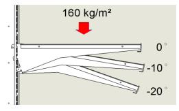
Do not exceed the loading capacity on pans and shelves. (160 kg / m<sup>2</sup>)
